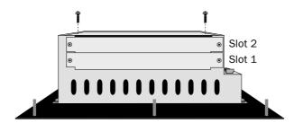
4. Put the jumper J1 on the expansion card in the position SLOT 1 if the expansion card is mounted in slot 1, and in position SLOT 2 if the card is mounted in slot 2.
